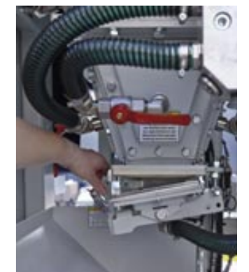
Maintenance flap at the filling box chamber
