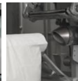
Spillage rejecting flap during bag discharge
