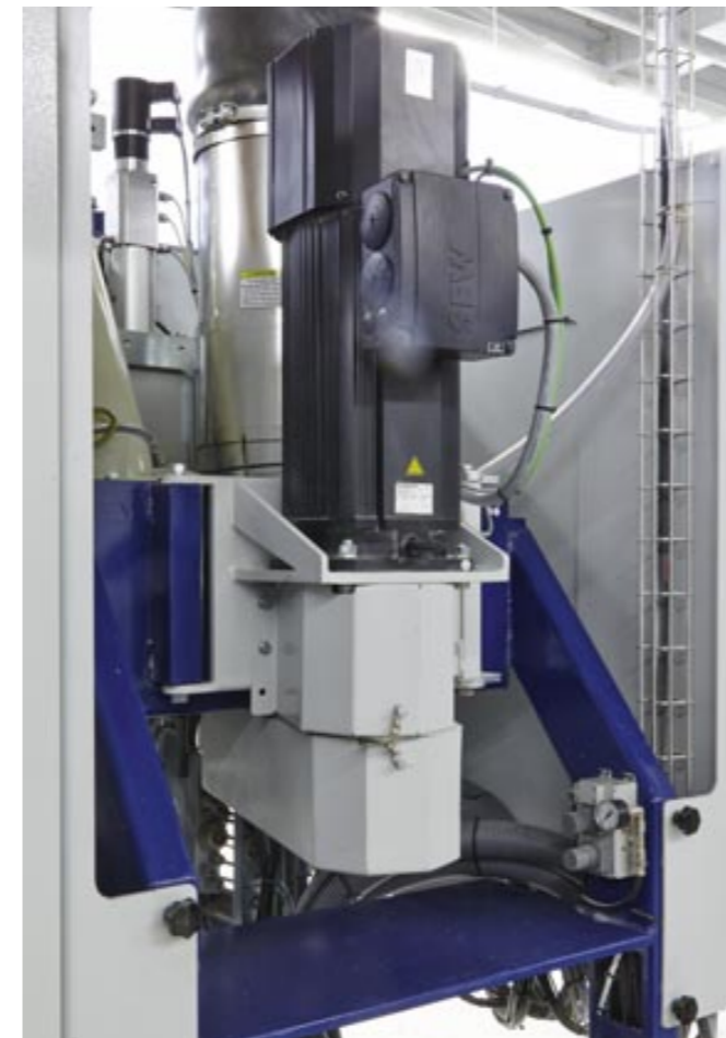
HAVER & BOECKER horizontal impeller with servo-drive
