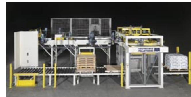
The palletizer - 4000 series - is used in the building materials industry and is suited for capacities of 2,500 - 4,000 bags/hr.
