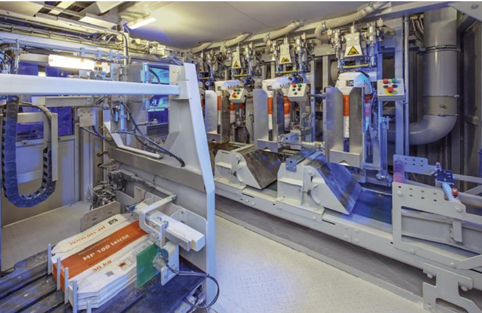
ELEMENTRA® with movable automatic bag placer - bundle system
