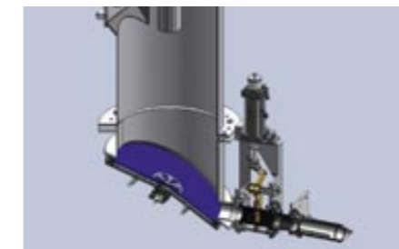
Conical valve in our inclined bottom air filling system
