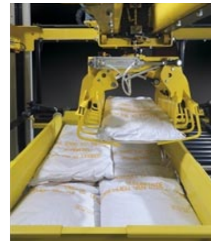
The palletizer - 4000 series - is used in the building materials industry and is suited for capacities of 2,500 - 4,000 bags/hr.
